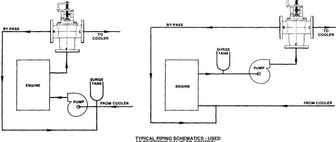
TYPICAL PIPING SCHEMATICS - USED AS DIVERTING VALVE TO CONTROL TEMPERATURE LEAVING ENGINE: PREFERRED AND MOST COMMON APPLICATIONS
