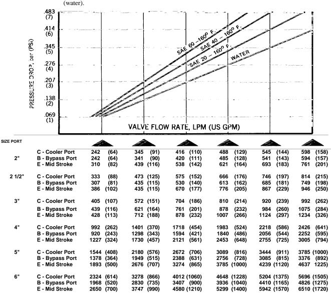
FLOW COEFFICIENTS: Table below indicates the flow in U.S. g.p.m. at different pressure drops.  $C_v$  Coefficients are listed in column 1 under .069 bar (1 psi) pressure drop
